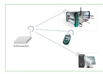
2. Connection of an ALMEMO® measuring device with an ALMEMO® WLAN module (client) to a WLAN network (access point in the company network)
