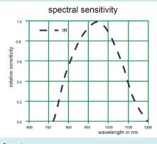
• This measures the solar spectrum in the short-wave IR range (excluding the visible range).
