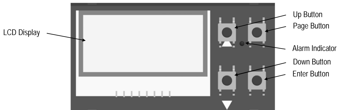
Figure 33: Control Panel for the Comm Box (DIN)
