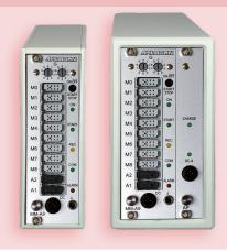
ALMEMO® precision measuring instrument for measured data acquisition, with data logger function. Comprehensive range of functions for all application areas. Increased measuring accuracy, fast measuring rate 9 measuring inputs.
