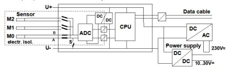
The 9 analog inputs are electrically isolated from one another by means photovoltaic relays. A new feature on this device is the <u>additional separation</u> of the measuring inputs from CPU and power supply. Between all inputs and outputs (even the analog output cables which are not electrically isolated) the maximum potential difference permitted is 50 V. The voltage at the measuring inputs themselves must not exceed 12 V (between B, C, D, and A).
