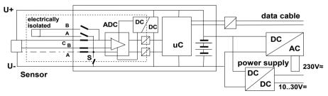
The analog inputs are electrically isolated from one another by means of photovoltaic relays. A new feature on this device is the <u>additional separation</u> of the measuring inputs from the CPU and power supply. Between all inputs and outputs (even the analog output cables which are not electrically isolated) the maximum potential difference permitted is 50 V. The voltage at the measuring inputs themselves must not exceed 12 V (between B, C, D, and A).
