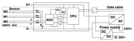
The analog inputs are electrically isolated from one another by means photovoltaic relays. A new feature on this device is the <u>additional separation</u> of the measuring inputs from CPU and power supply. Between all inputs and outputs (even the analog output cables which are not electrically isolated) the maximum potential difference permitted is 50 V. The voltage at the measuring inputs themselves must not exceed 12 V (between B, C, D, and A).
