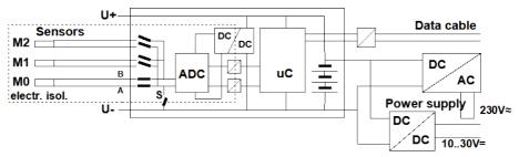
The 9 analog inputs are electrically isolated from each other by means of photovoltaic relays and - on this device for the first time - also from the device itself and from the power supply by means of optocouplers. Between all inputs and outputs (even the analog output cables which are not electrically isolated) the maximum potential difference permitted is 50 volts. The voltage at the measuring inputs themselves must not exceed 12 volts (between B, C, D, and A).
