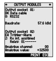
With the relay trigger analog modules certain function variants can be configured (see 11.6.2), relays can have certain limit values assigned to them, or analog outputs can be assigned to certain measuring channels. In this menu all ports can be selected and configured accordingly. The connection possibilities are described in the instructions for the output module concerned.
