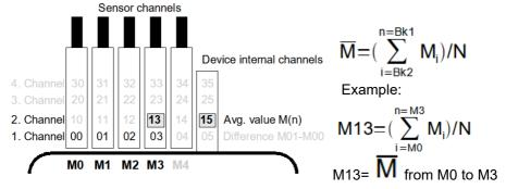
If the sensors are to stay untouched, the function channel can also be programmed to the device internal channels (e.g. M15) (s. 11.3.10). The standard reference channels are here M0 to M1.
