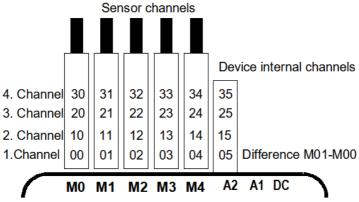
programmed by default as differential channel M1-M0; this applies if there are two sensors with the same units and same decimal point position connected at measuring points M0 and M1. However, all four channels can be used in conjunction with any function channels with standard reference channels Mb1=M1 and Mb2=M0 assigned; i.e. if you want to program a function parameter without reference channel on a device-internal basis, the sensor must be connected to M1.
