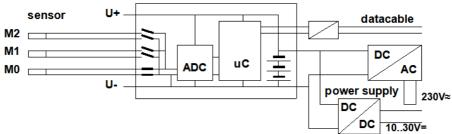
The analog inputs are electrically isolated by means of photovoltaic relays; the maximum potential difference permitted between them is 50 VDC or 60 VAC. Sensors combined within one connector and sensors with their own power supply, however, are electrically interconnected and must therefore be operated in
