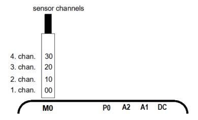
Sensors combined within one connector and sensors with their own power supply are electrically interconnected and must therefore be operated in isolation. The voltage at the measuring inputs themselves must not exceed 5 volts (between B, C, D, A and - ).
