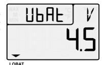
The measured value is then displayed with the appropriate units in the main field and the measuring point is displayed in the function field. All special operating states possible for the measured value are explained in Section 9.1.
