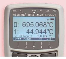
Reference measuring instrument for temperature.
