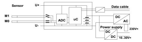
The analog inputs are electrically isolated by means of photovoltaic relays; the maximum potential difference permitted between them is 50 VDC or 60 VAC. The power supply is isolated by the transformer in the mains adapter or by a DC/DC converter in connecting cable ZA2690-UK.
