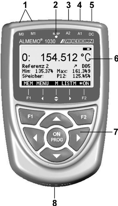
(1) **Measuring inputs M0 and M1**
