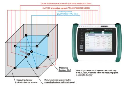
Humidity is calculated in the ALMEMO<sup>®</sup> 710 on the basis of formulae as per Dr. Sonntag and the enhancement factor as per W. Bögel (correction factor Fw(t,p)) for real mixed gas systems). This substantially widens the measuring range and improves the accuracy of humidity variable calculations.
