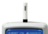
ALMEMO® 2790 with sensors for humidity, temperature, atmospheric pressure option OA 2790-RHA
