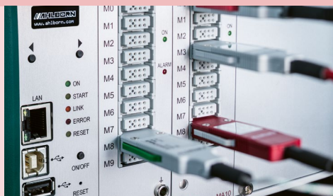
Ports for ALMEMO® sensors and for networking (OLED status display)
