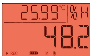
Automatic alarm (red background). Display shows incorrect measured value
