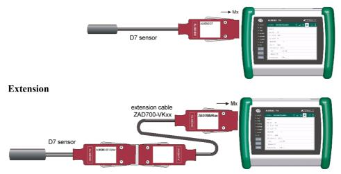
The operating radius of these sensors when connected to a measuring instrument can be extended by means of extension cable ZAD700-VKxx; measured values and connector programming can then be transmitted interference-free in serial form via an RS-422 driver. For electrical isolation adapter cable ZAD700-GT can be used.
