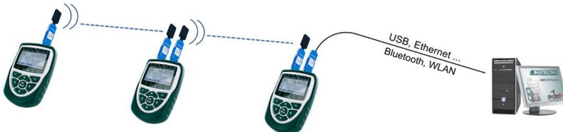
**new: Wireless connection between ALMEMO® measuring instrument via Bluetooth**
