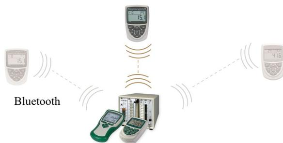
**Wireless sensor connection via Bluetooth (ALMEMO® wireless sensor)**
